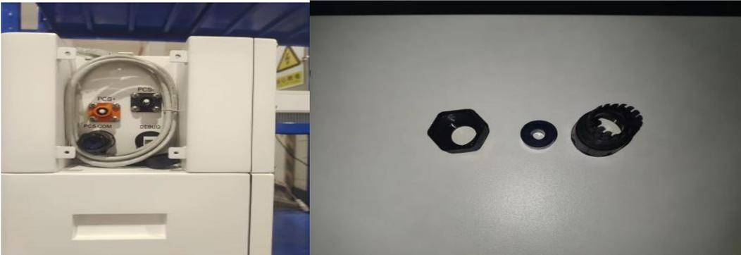
3. Assemble one end of the waterproof pair connector and the communication cable in the sequence shown in the following figure and tighten it. After connecting to the PCS COM port, tighten the waterproof pair connector (you can directly insert the network cable without connecting the waterproof head during indoor wiring). Connect the other end of the network cable to the BMS port of the inverter.
