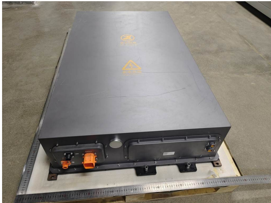
Side view of battery module (with MSD)
