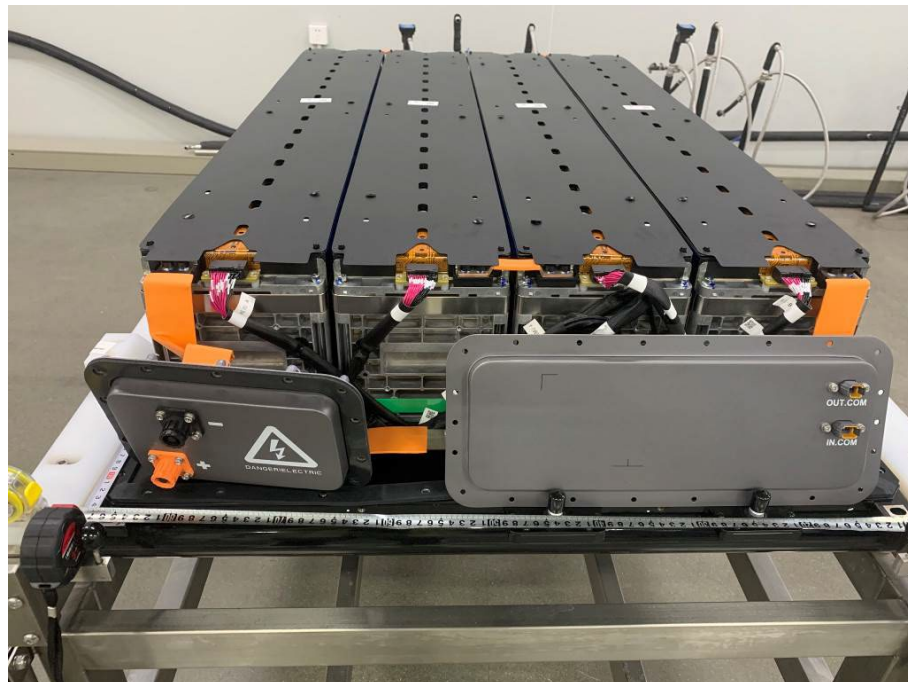
Inside view of battery module (without MSD)
