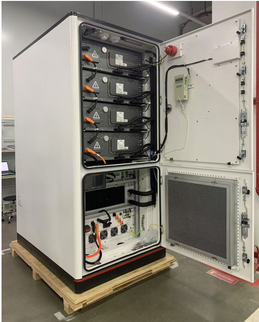
Inside view of battery system (without MSD)
