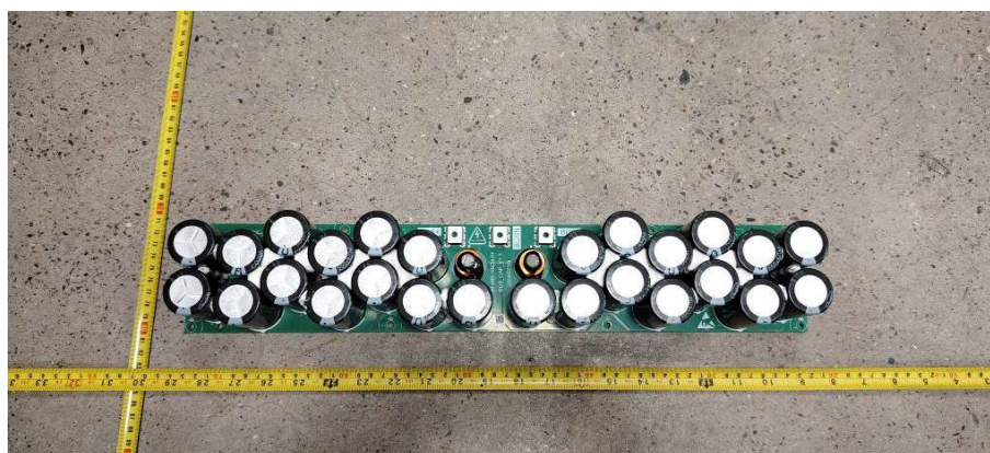
Bus capacitor board of PCS
