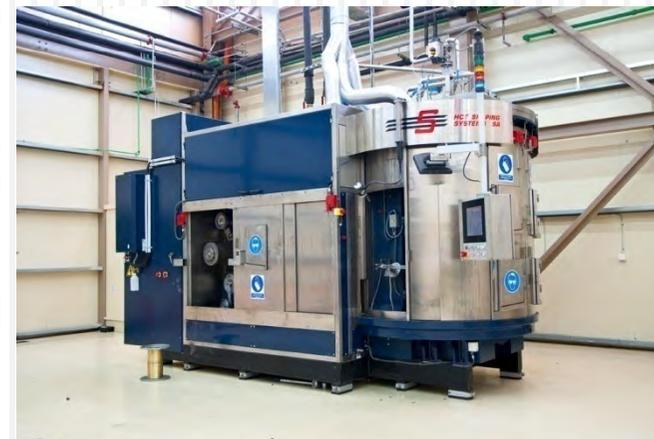
**Key facts: Production of thinner wafers, reducing kerf loss, recycling cutting slurry in house.**
