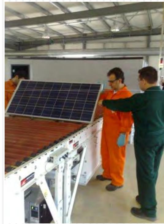
**Key facts: Automated production, mechanical load up to 5400Pa**
