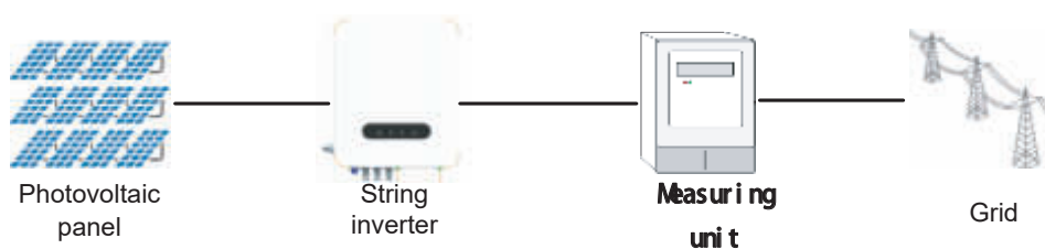
Figure 2-6 Application diagram of the string inverter network
