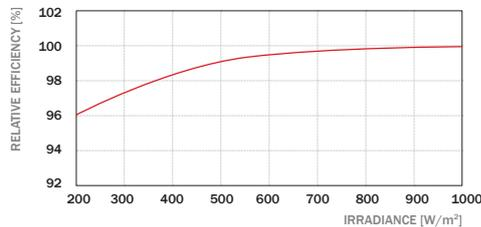
The typical relative change in module efficiency (with respect to nominal power) at an irradiance of 200 W/m<sup>2</sup> in relation to 1000 W/m<sup>2</sup> (both at 25 °C and AM 1.5 G spectrum) is -4.0 % rel.
