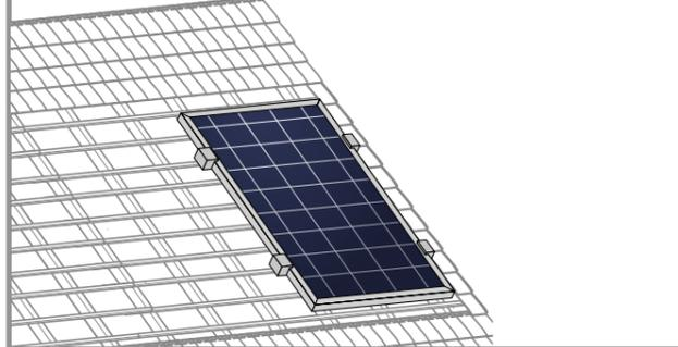
→ Maintain an interval of at least 10 mm between two modules along the short side and 5 mm along the long side.
