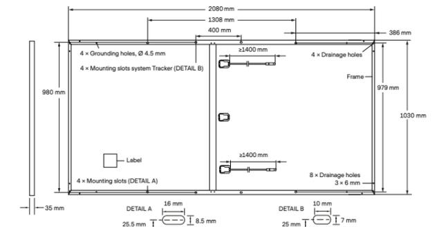
**Fig. 2:** External dimensions (in mm) and components for Q.PEAK DUO L-G8.1, Q.PEAK DUO L-G8.2,
