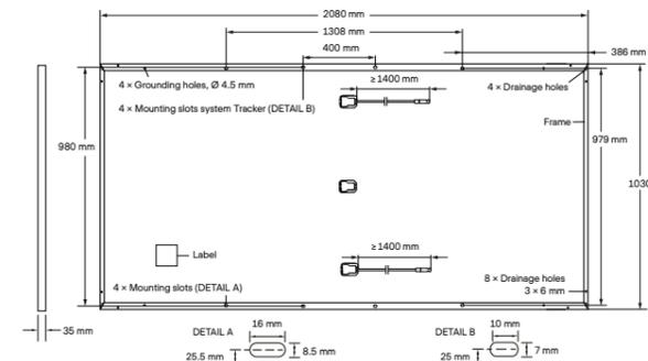
**Fig. 1:** External dimensions (in mm) and components for Q.PEAK DUO L-G8, Q.PEAK DUO L-G8.3,
