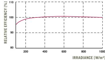
The typical change in module efficiency at an irradiance of 200 W/m<sup>2</sup> in relation to 1000 W/m<sup>2</sup> (both at 25 °C and AM 1.5 G spectrum) is -2.5% (relative).
