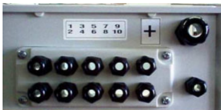
Figure 9-18: Cable gland for positive strings connection
