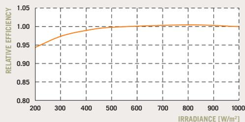
The typical relative change in module efficiency at an irradiance of 200 W/m<sup>2</sup> in relation to 1000 W/m<sup>2</sup> (both at 25 °C and AM 1.5 spectrum) is less than 6 %.
