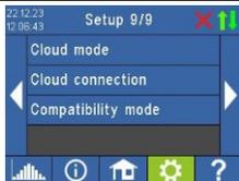
If desired, the settings of the AC ELWA 2 can also be accessed from outside the local network. For this purpose, it is necessary to register the device with serial number and device key in the my-PV Cloud: <https://live.my-pv.com/>
